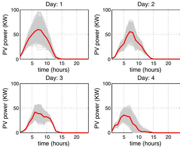
Fig. 2. PV power output for four representative days. For each day, the “red” curve corresponds to the forecast, whereas the “gray” curves show the forecast plus the forecast errors.
