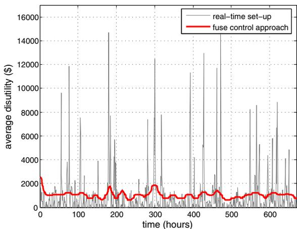
Fig. 5. Average disutility due to load curtailment for the fuse control (“red”) and real-time (“gray”) price set-up.
